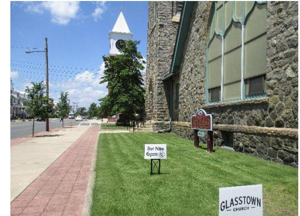
Parking spots east of the parking lot can be replaced with porous asphalt to capture and infiltrate stormwater. The sidewalk at the entrance of the church can be made porous to capture, treat, and infiltrate roof runoff. A preliminary soil assessment suggests that the soils have suitable drainage characteristics for green infrastructure.
