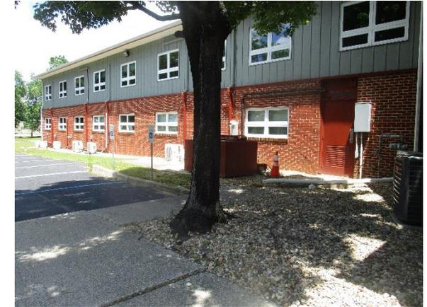
Parking spots in the north section of the parking lot can be replaced with porous asphalt to capture and infiltrate stormwater. A rain garden adjacent to the building can capture, treat, and infiltrate roof runoff. Planter boxes and rainwater harvesting systems can collect additional runoff and beneficially reuse it. A preliminary soil assessment suggests that the soils have suitable drainage characteristics for green infrastructure.
