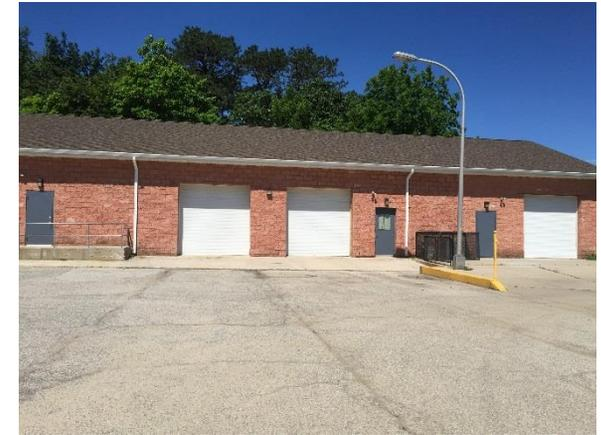
Parking spots can be replaced with porous asphalt to capture and infiltrate stormwater. Rain gardens at the entrance and near the sports fields can capture, treat, and infiltrate roof runoff. Planter boxes can collect rain water from the roofs and beneficially reuse it. A preliminary soil assessment suggests that the soils have suitable drainage characteristics for green infrastructure.
