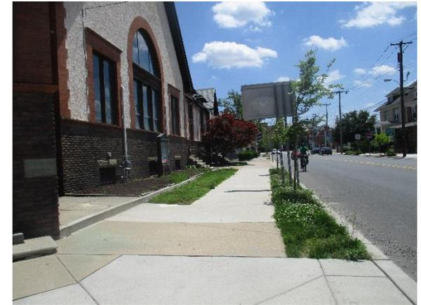
Pervious pavement such as pervious sidewalk can be implemented on the north side of the building which can capture, treat, and infiltrate roof runoff. A preliminary soil assessment suggests that the soils have suitable drainage characteristics for green infrastructure.
