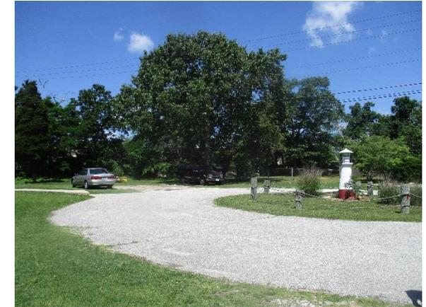
Parking spots to the north of the parking lot can be replaced with porous asphalt to capture and infiltrate stormwater. A rain garden in the middle of the parking circle north of the building can capture, treat, and infiltrate roof runoff. A preliminary soil assessment suggests that the soils have suitable drainage characteristics for green infrastructure.
